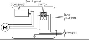
Three-phase motors are supplied with a terminal strip box and terminal strip. To connect the electric motor to the electric power line, open the terminal strip cover and connect the cables according to the diagram.
