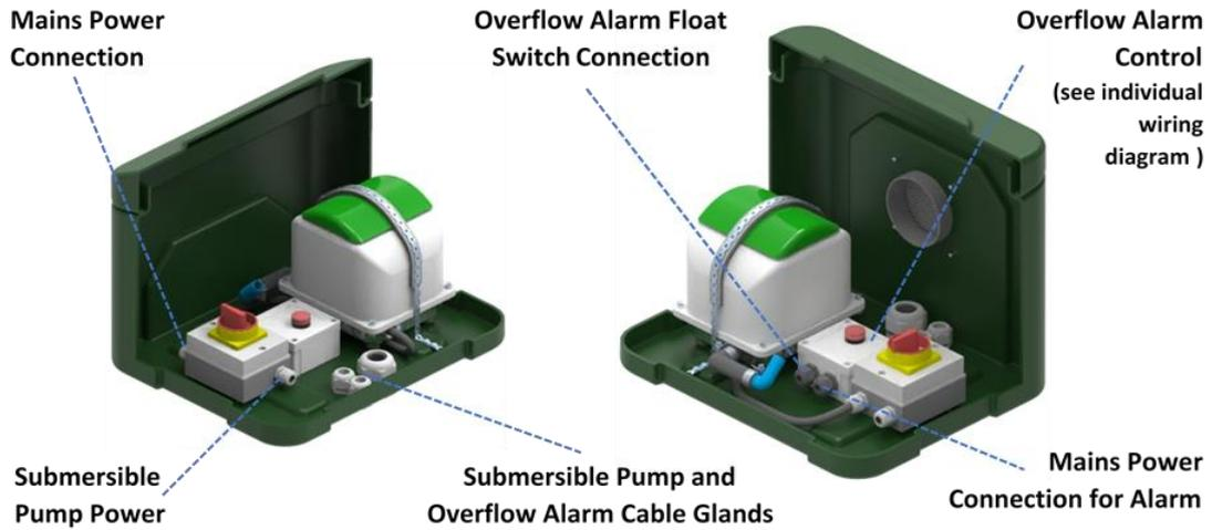
Figure 9: External Blower box assembly (Pumped Outlet version)
