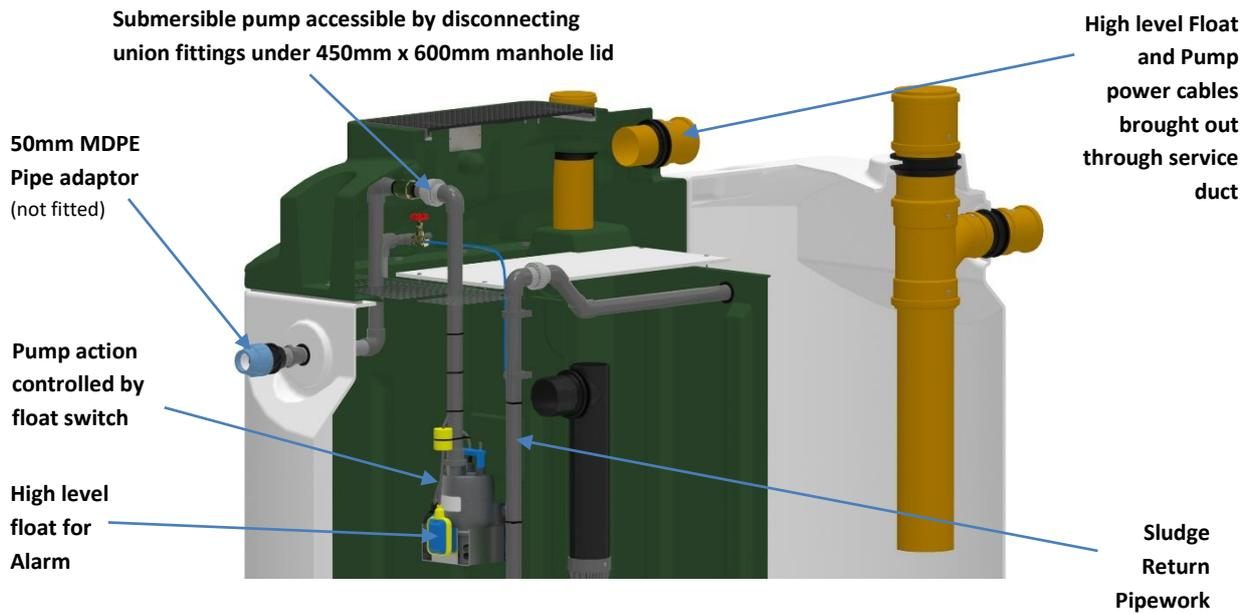
Figure 7: Tank Configuration in Pumped Outlet version
