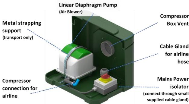
**Figure 5:** Inside the External Air Blower Housing
